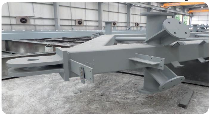
Complex Designed, Detailed & Fabricated Steel to Steel Connections
